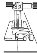
Match the finished line, needle position, and guide A, then sew.
