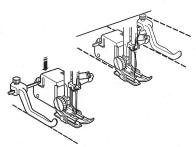
Ditch quilting guide aligns with center of foot for ditch quilting or top stitching.
