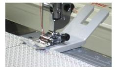
2. Start sewing; remove the plate once the foot is fully on the fabric.
