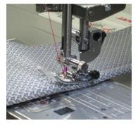
2. Lift the foot, gently push on front of the foot to make it level, then push the button in to lock it into posiiton.
