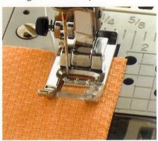
If using the center needle position, align the fabric edge slightly to the left of the 2mm marking on the needle plate.
