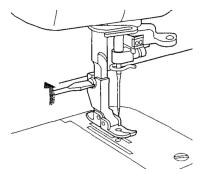
3. Attach the 2mm Bi-level Spring Action Guide foot and tighten the screw.
