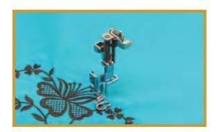
**Note:** Be sure to use Embroidery Foot "W" when doing embroidery. Using another presser foot may cause the needle to strike the presser foot, causing the needle to bend or break and possibly cause injury.
