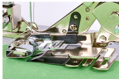
Base fabric under Separator Blade.
