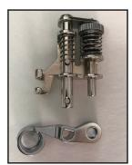
b. Align the flat side of the freemotion foot shank with the flat side of the hole in the sole. The base of the presser foot height adjustment post must also fit into the small indentation in the sole.
