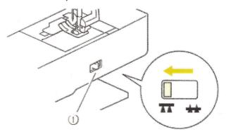
7. Check your machine settings and make sure Free-Motion mode is set to "ON". The default setting "OFF" is selected.
