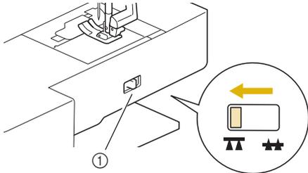
① Feed dog position switch (as seen from the rear of the machine)
