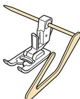
2 Adjust the stem of the quilting guide so that the guide aligns with the seam that has already been sewn.
