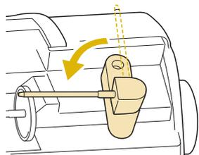
**6** Place the upper thread spool for the needle on the right side onto the horizontal spool pin, and then secure it with the spool cap.
