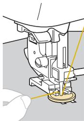
→ The machine automatically stops after sewing reinforcement stitches.
