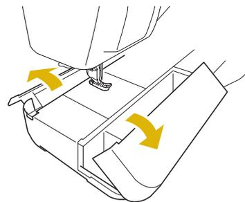
A presser foot accessory tray is stored in the accessory compartment of the flat bed attachment.
