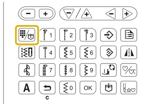
2 Press the numeric key on which the desired stitch is printed.
