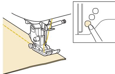
→ The machine stops with the needle in the fabric, and the presser foot is raised.
