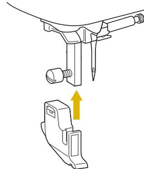
**3** Hold the presser foot holder in place with your right hand, and then tighten the screw using the screwdriver in your left hand.
