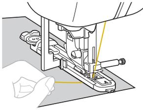
→ Once sewing is completed, the machine automatically sews reinforcement stitches, then stops.
