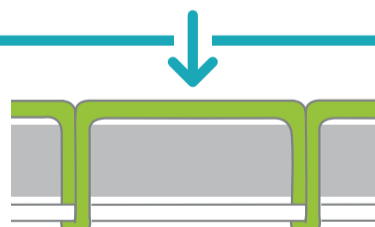
Top tension is too LOOSE .
